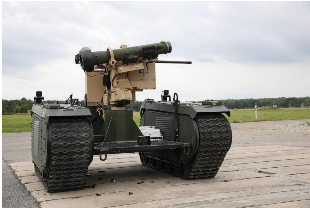
QinetiQ Titan robot fitted with a Javelin anti-tank missile launcher.
