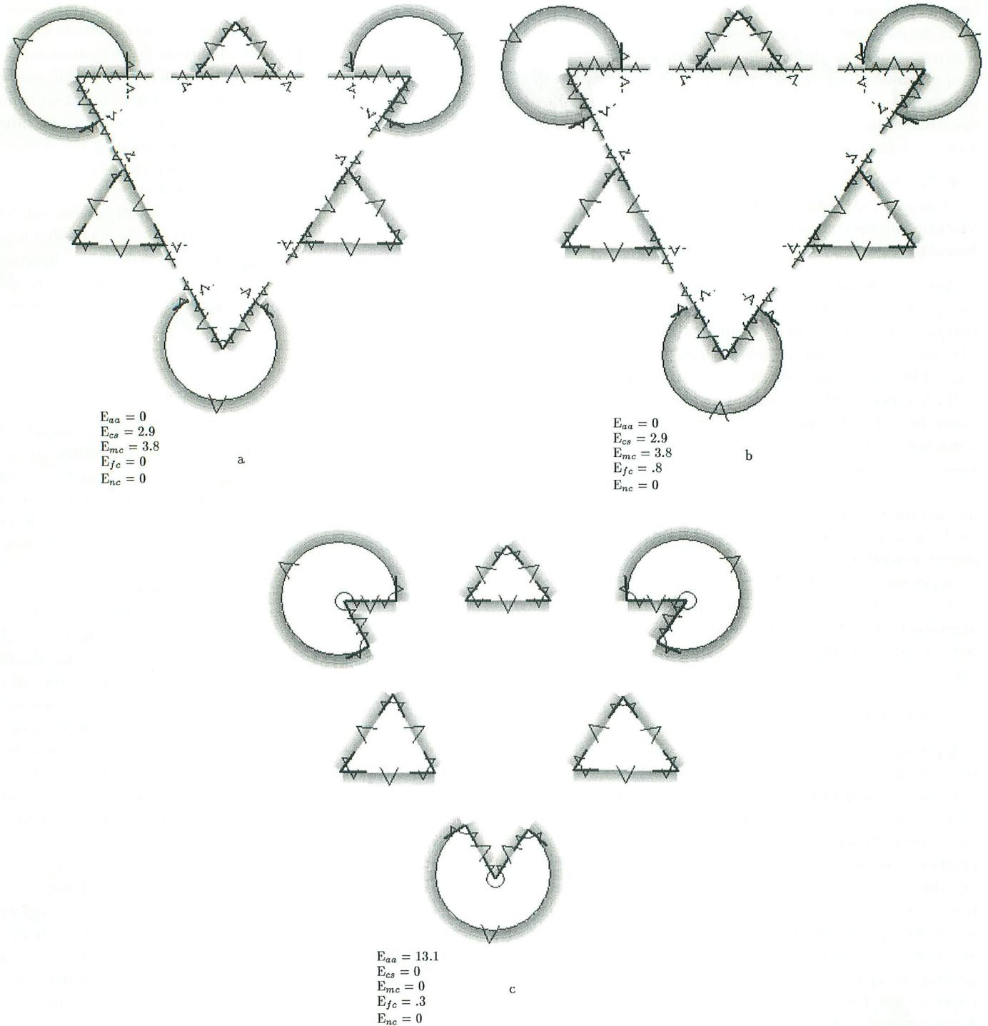
FIG. 9. Three among many possible interpretation labelings of the Kanizsa triangle and their associated energy costs. All labelings are stable at high inverse-temperature, but a (the global optimum) is converged to by the algorithm annealing from low inverse-temperature. Shading resembling shadowing is added to enhance visualization of program output.
