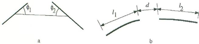
FIG. 16. a. The angles  $\phi_1$  and  $\phi_2$  used to measure the alignment of two boundary contour ends. b. The lengths  $l_1$ ,  $l_2$ , and  $d$  used to measure the scale-normalized distance between the ends of two boundary-contours.
