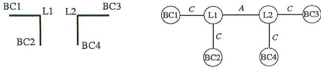
FIG. 10. Four BOUNDARY-CONTOURS forming two L-JUNCTIONS and their corresponding junction-graph containing coincidence links (C) and an alignment link (A).
