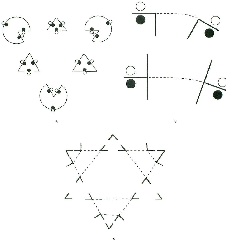
FIG. 11. a. BOUNDARY-CONTOURS tokens for the Kanizsa triangle figure. b. Alignment links are created between pairs of L-JUNCTION legs and pairs of T-JUNCTION stems that are sufficiently near and aligned with one another and whose bounding surface colors match. c. L-JUNCTIONS (solid lines) and alignment links (dashed lines) found for the Kanizsa Triangle figure.
