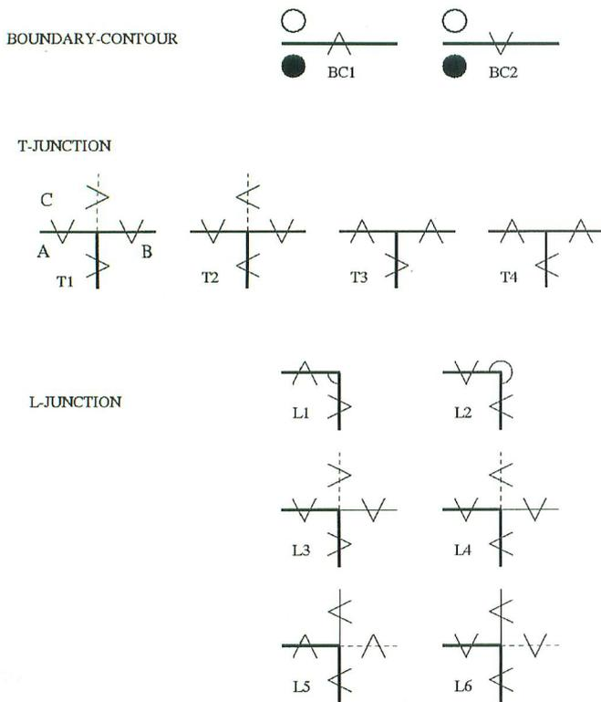
FIG. 3. Catalog of interpretation labels for BOUNDARY-CONTOURS, T-JUNCTIONS, and L-JUNCTIONS. Heavy lines denote contrast edges, solid thin lines denote modal completion contours, dashed lines denote occluded contours. Arrows indicate direction of surface overlap; tip of arrow indicates *occluded* surface.
