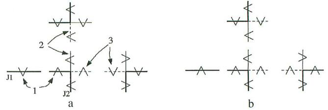
FIG. 12. a. An incompatible assignment of junction labels due to: (1) incompatibility between an L-JUNCTIONS and one of its associated BOUNDARY-CONTOURS; (2) incompatibility between modal completion and amodal contour continuation interpretations; (3) incompatibility between overlap directions across an amodal continuation link. b. A compatible assignment of junction labels.
