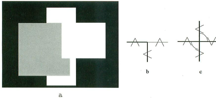
FIG. 5. a. The interpretation of a white square overlapping and aligning the grey square requires a junction label of nongenericity degree 2, shown in b, due to accidental edge alignment and surface color match. c. An X-junction label, nongenericity degree 2, due to double accidental edge alignment. The algorithm implemented limits itself to junctions of nongenericity degree 0 and 1.
